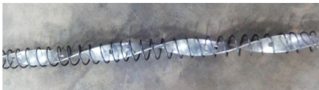
Fig.3: Photograph of the combination of porous twisted tape with wire coil
